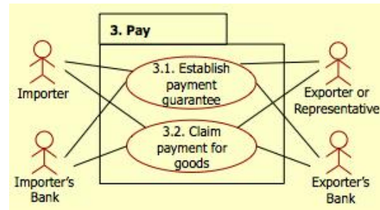
Figure A3-28. Use case diagram of core business processes in pay process area
